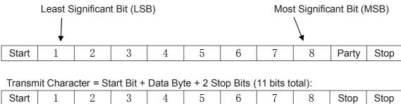
Eastron Digital meters additionally support No parity, One stop bit.
